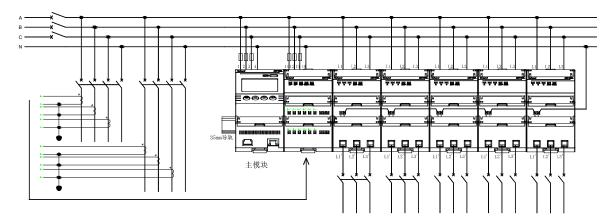
2 channels of transformer access + 2 channels of three items direct access + 6 channels of single item direct input
